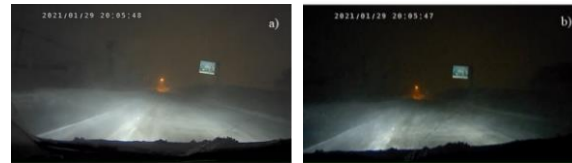
Captured images are taken by the industrial camera during the observation. The exposure time is a) auto, b) 40ms
