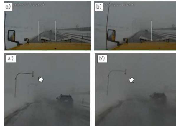
Captured images are taken by the industrial camera. The exposure time is a) 0.16ms, b) 40ms
