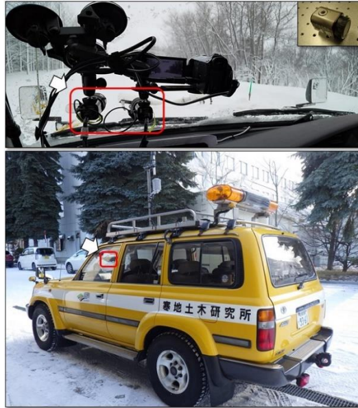
Figure 1. Weather observation vehicle (lower image) and industrial cameras lined up on the windshield (upper image). An image of the industrial camera shows up-right corner of the upper image.
