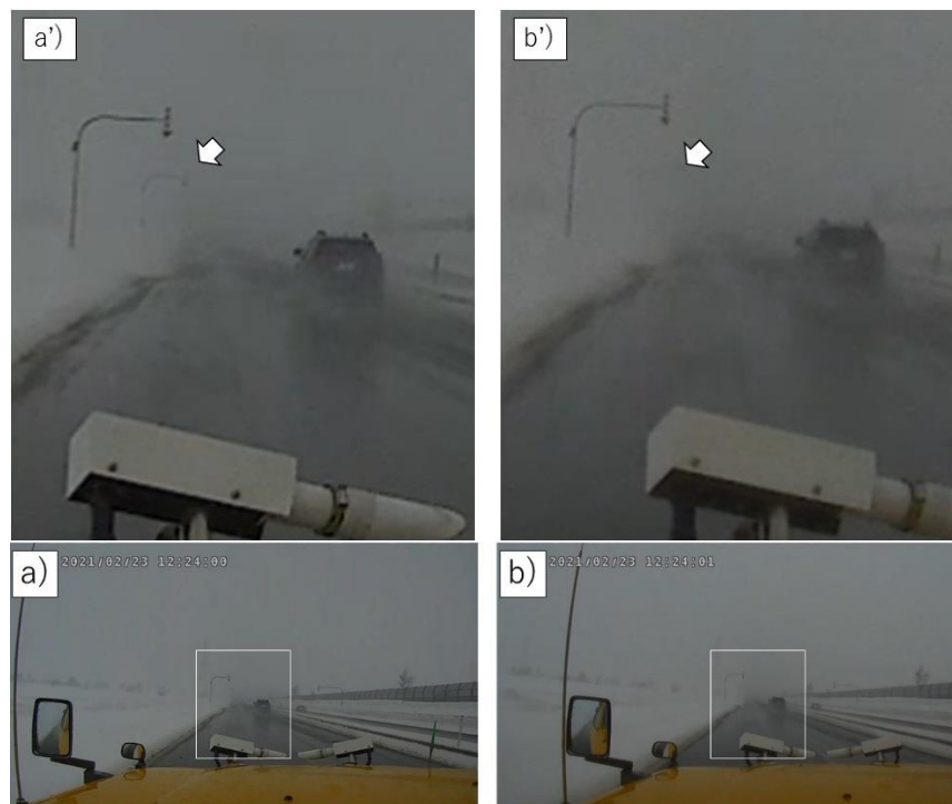
Figure 2. Captured images are taken by the industrial cameras lined up on the windshield of the weather observation vehicle. The exposure time is a) 1/6400 second and b) 1/25 second, respectively. a') and b') are enlarged images of the white frames in a) and b), respectively. The arrows in the figures indicate a fixed-post delineator located 50 m distant from the forefront delineator.
