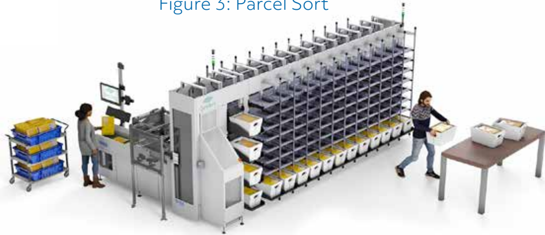
Figure 3: Small parcels can be sorted to the zip code level for shipping efficiency and to reduce costs.
